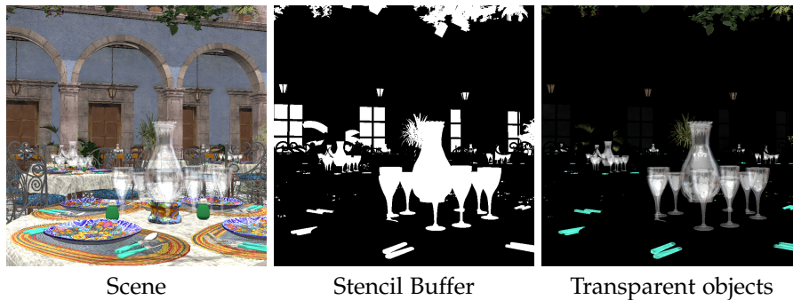
Figure 4.9: The stencil buffer is used to create a mask from transparent object.
